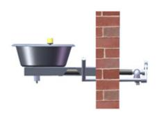
Size Eye wash model MBS30 DDM (stainless steel)Article number999999979MaterialStainless steel bath, chrome plated brass nozzlesPipeworkRVSOperationStainless steel push handleWater flow12 l/min. (2 Bar G)Water supply15 mm compression fitting, ½" BSP external thread
